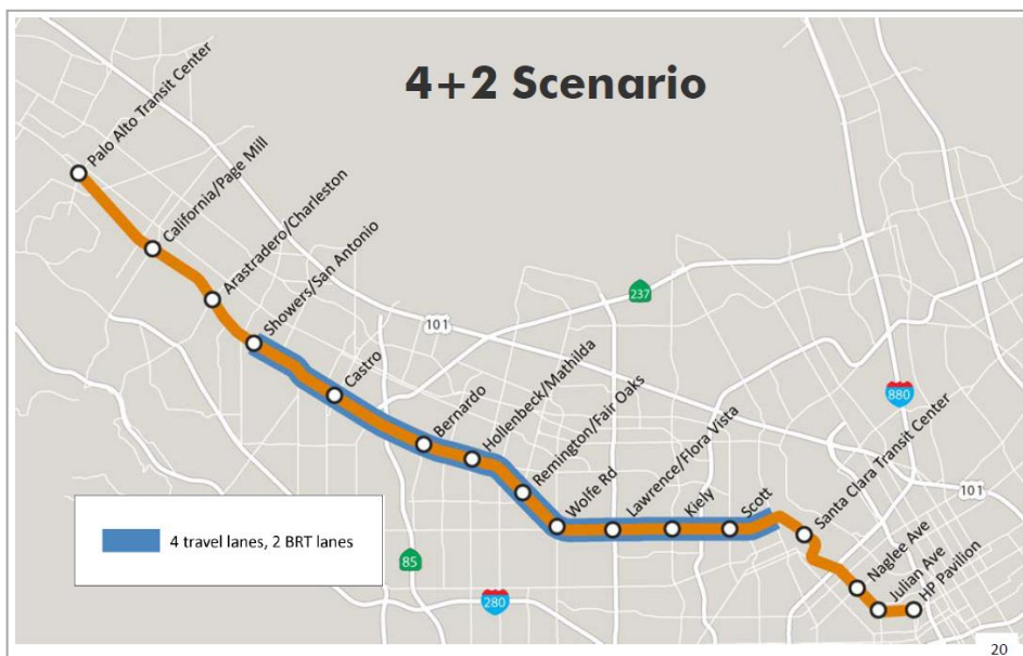
BRT will better-connect the downtowns of Palo Alto, Mountain View, Sunnyvale, and San Jose, as well as Stanford and Santa Clara Universities. The area highlighted in blue is proposed for exclusive bus lanes. Image source: www.valleyrapid.org
