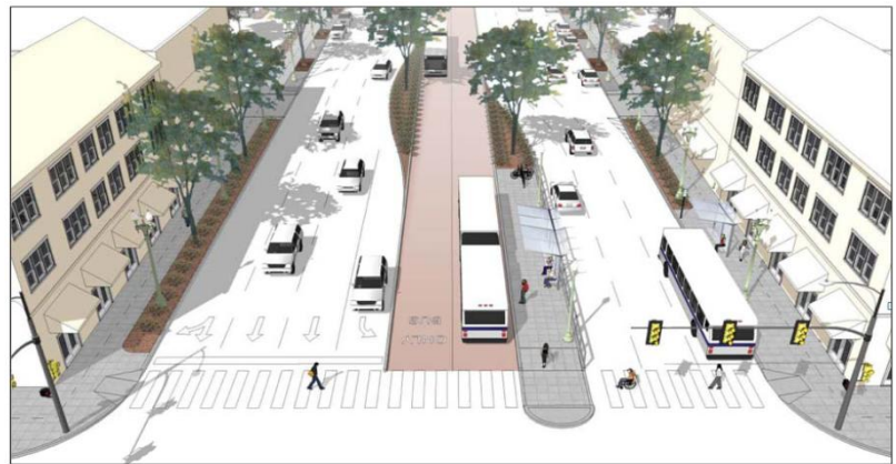
Signalized left turn lanes can be preserved: An illustration of a northbound BRT station with exclusive bus-lanes and left turn lanes. Image source: www.valleyrapid.org
